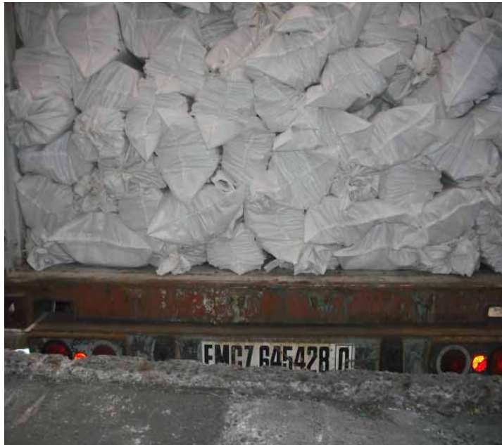
Figure 5-5-8 Example of Inadequate Spacing Under Bamboo Bundles
