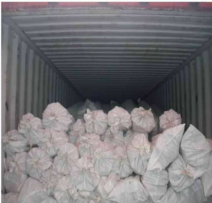
Figure 5-5-10 Example of Adequate Space Above the Bamboo Bundles
