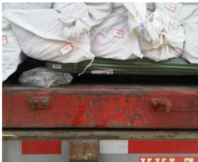
Figure 5-5-9 Example of Inadequate Spacing Under Bamboo Bundles
