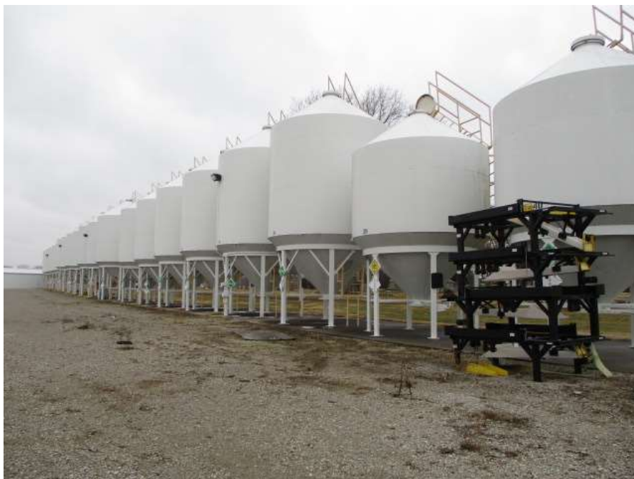
Freisen/Meridan (white powder coat) hopper bottom storage bins – on north property line
